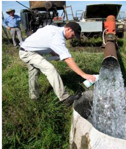
Taking a water sample for Laboratory analysis
